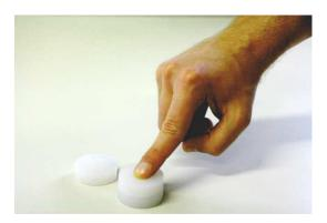
Figure 7. A subject's hand palpating one of the silicone specimens used in the tests.
