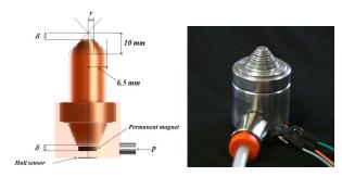
Figure 4. Geometry (left) and appearance (right) of the softness display. The prototype has a max. height of 33 mm and a diameter of 13 mm.
