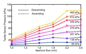
Fig. 4. Tactile sensor measurement results. Each data point represents the peak output pressure value measured on the tactile sensor array for a particular air supply pressure and aperture size. Numbers at right represent supply pressures (rounded). Line styles indicate order of supply pressures used in measurement.
