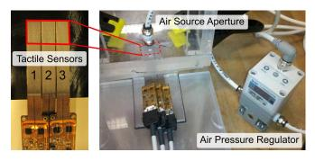
Fig. 2. Setup for tactile sensor measurement. The air pressure regulator connects directly to the air source aperture and controls supply pressures. Tactile sensors placed under the aperture record distributed pressure as supply pressure and aperture size are varied.
