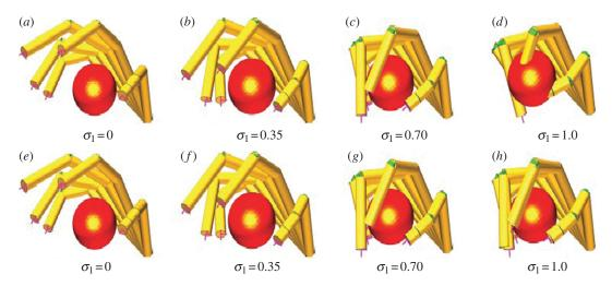
Figure 3. In the soft synergy model, the reference hand moves on the synergy manifold (a-d) and represents an attractor for the real hand (e-h), which is repelled by contact forces with the object. The resulting configuration is ultimately dictated by the hand mechanical and control stiffness.
