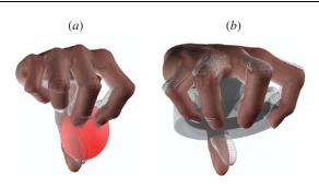
Figure 4. Application of the soft synergy model to the grasp of a cherry-like object (a) and of an ashtray (b). In wireframe is the reference hand, moving according to the constraint manifold corresponding to the first three synergies.
