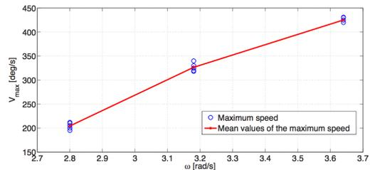
Fig. 9. Constrained terminal time problem: experimental maximum velocity obtained for a fixed terminal time and several stiffness values.
