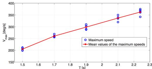
Fig. 8. Constrained terminal time problem: experimental maximum velocity obtained for a fixed stiffness value and several terminal times.
