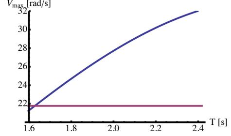
Fig. 6. The blue line represents the final speed of the VSA for the constrained terminal time problem ( $u_{\max} = -u_{\min} = \pi \text{rad}$ ,  $\omega_{\max} = 2.5 \text{rad/s}$  and  $\omega_{\min} = 1 \text{rad/s}$ ). The red line represents the final speed for the SEA in case of unconstrained terminal time problem ( $u_{\max} = -u_{\min} = \pi \text{rad}$  and  $\omega_{\max} = 2.5 \text{rad/s}$ ).
