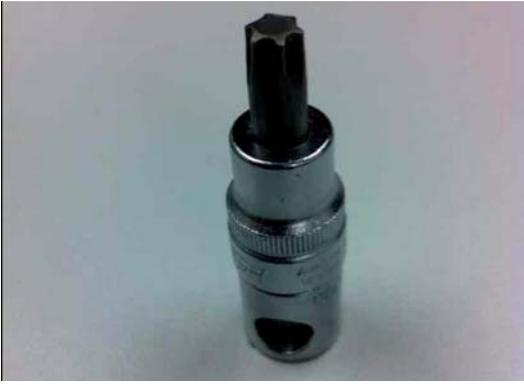
Fig. 16. Torx 45: a typical industrial end-effector tool.
