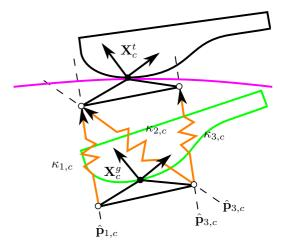
Fig. 3. Representation of the spatial spring placed at the contact locations. In this planar case, the contact model is SF, hence there are  $h_c=3$  linear springs. The triangles are drawn for clarity, however, the vertices coincident with the contact point, making  $\mathbf{p}_{1,c}, \mathbf{p}_{2,c}$  and  $\mathbf{p}_{3,c}$ , pass through the origin of  $\mathbf{X}_c$ . The rest position of the springs correspond to the configuration where  $\mathbf{X}_c^g = \mathbf{X}_c^t$ .
