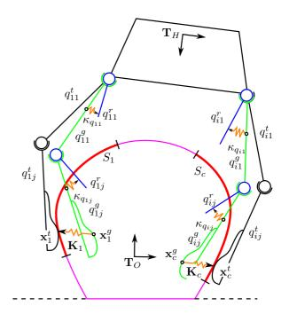
Fig. 2. Kinestatic model using springs at the joints and at the contact. The grasp is characterized by three hand configurations accounting for the feasibility and prehensility of a grasp.
