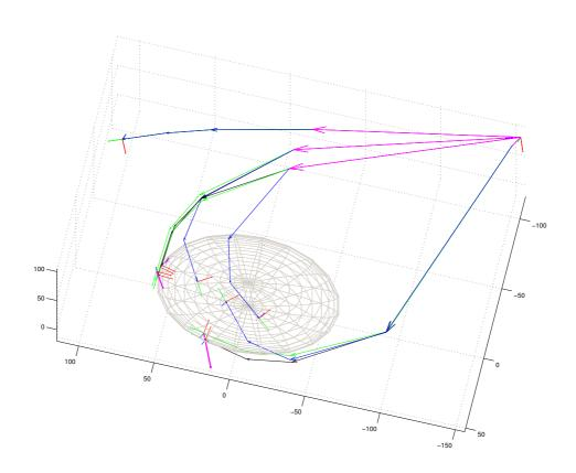
Fig. 5. A solution obtained for the Schunk Anthropomorphic hand satisfying all constraints performing the grasp with three fingers.
