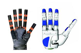
Fig. 1. Different multi-fingered robotic hand designs. The left image corresponds to THE first hand developed at the Centro E. Piaggio with five fingers, and the right image corresponds to the Schunk Anthropomorphic hand, based on the DLR II hand, with four fingers
