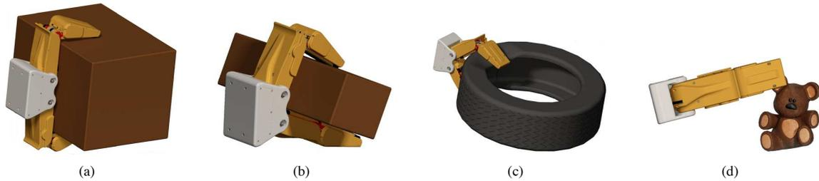
Fig. 17. Examples of grasps obtained with the "velvet fingers" dexterous gripper. Grasped objects are part of the scenario of the EU founded project ROBLOG ([www.rob1og.eu](http://www.rob1og.eu)), for which this EE has been designed. The objects grasped are: a big box 390x290x270mm (a), a small box 376x149x122 mm (b), a tire P195/55R16 85H (c) and Teddy bear (d).
