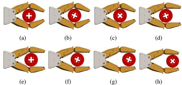
Fig. 5. Manipulation enhancement by using pushing active surfaces. Pictures show how the grasped object can be rotated (a, b, c, d), translated (f, g), or simultaneously rotated and translated (e, h), combining the two movements.
