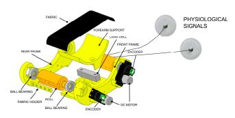
Fig. 1: The main components of the affective haptic device and the envisaged front end for the acquisition of the physiological signals from the user.
