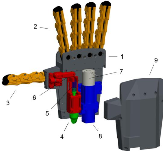
Fig. 3. CAD Model of the prototype of the dynamic synergies hand. The viscous element is placed in the dorsal side of the palm, directly connected with the distal and proximal joints of the thumb.
