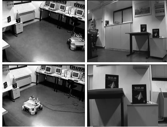
**Fig. 1.4** External views (left column) and subjective images (right column) as taken from the vehicle, in the initial configuration (top row) and in the final configuration (bottom row), after reaching convergence under the proposed visual feedback control scheme. The bottom right image should be compared with the target image in fig. 1.3.
