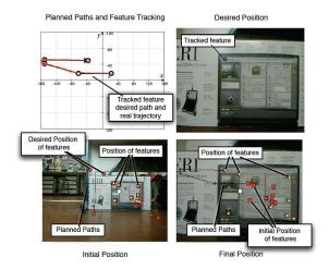
Fig. 9. Experiment 2. Planned paths and trajectory of the tracked feature (up left). Initial (bottom left), final (bottom right) and desired (up right) images taken from the vehicle. The initial and desired positions of the features are plotted over the initial and final images taken from the vehicle. The actual positions of the features are also shown in these images.
