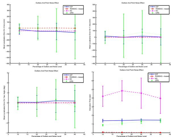
Fig. 1. Accuracy on the  $X_w$  and  $Y_w$  axis (in millimeters, upper row), accuracy of the orientation angle (in degrees, bottom row, left) and the execution time (in seconds, bottom row, right). The effect of both noise (drawn from a Gaussian distribution with increasing standard deviation from 0mm to 40mm) and outliers (with a percentage from 0% to 40%) are reported.
