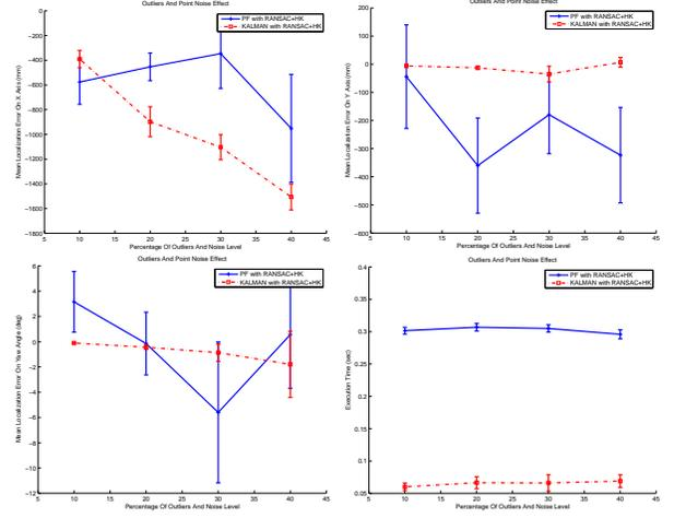
Fig. 3. Accuracy on the  $X_w$  and  $Y_w$  axis (in millimeters, upper row), accuracy of the orientation angle (in degrees, bottom row, left) and the execution time (in seconds, bottom row, right). The effect of both noise (drawn from a Gaussian distribution with increasing standard deviation from  $0mm$  to  $40mm$ ) and outliers (with a percentage from 0% to 40%) are reported.
