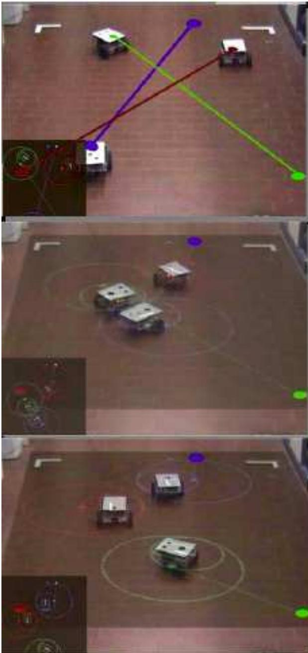
Fig. 16. Example of collision avoidance component experimental results.
