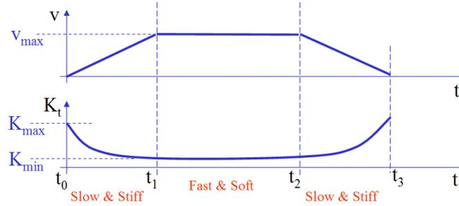
**Fig. 5.** Illustrating the intuitive behaviour of a Variable Stiffness Transmission in a 1DOF rest-to-rest task. High stiffness is imposed at low velocities, while transmission compliance is introduced at high velocities to reduce potential impact injuries.
