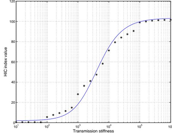
**Fig. 3.** Head Injury Coefficients evaluated for the impact of a link of effective inertia  $M_{link} = 0.1 \text{ Kg}$  elastically coupled to a rotor of inertia  $M_{rot} = 1.2 \text{ Kg}$  by a transmission with  $B_{transm} = 0$ , as  $K_{transm}$  varies. The rotor and link are assumed to move uniformly at velocity  $v = 10 \text{ m/s}$  before impact.
