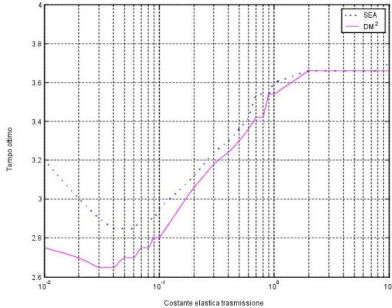
**Fig. 4.** Minimum time to goal under safety constraints and actuator saturation, as a function of the elastic coupling stiffness, for a passive elastic joint (dashed) and for a  $DM^2$  actuation scheme.
