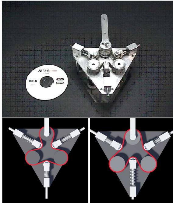
**Fig. 8.** (top) Appearance of the prototype VS actuator being developed at Centro “E. Piaggio”, University of Pisa. (bottom) The VS actuator in compliant (left) and stiff (right) configuration.
