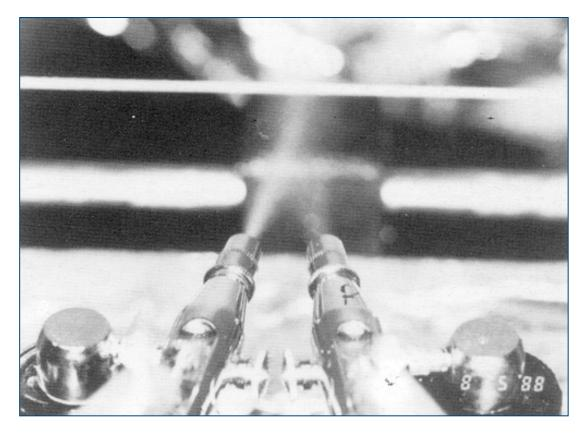
Two modified spray guns were mounted on the carriage and positioned vertically so that their nozzles were aligned with the longitudinal axis of the mandrel, at the distance and an angle from the mandrel such that the intersection of the jets occurred at the surface of the mandrel.
