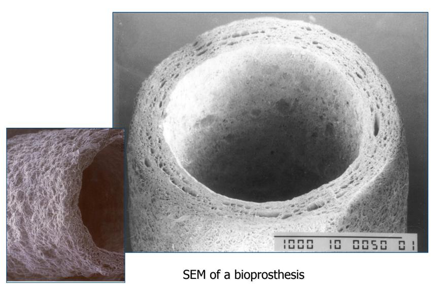
(SEM of the small diameter vascular graft (internal diameter 1.5 mm)
