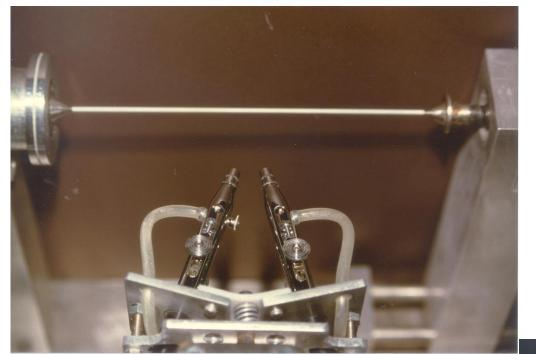
To fabricate the prostheses, we designed and built a small precision lathe in which mandrels of different diameters could be rotated at different speeds.
