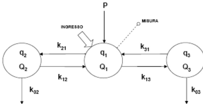
$$\dot{q}_1(t) = -(k_{21} + k_{31})q_1(t) + k_{12}q_2(t) + k_{13}q_3(t) + d\delta(t)$$
