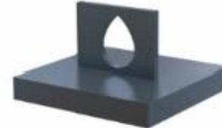
If the hole has an angled or arched upper area it will probably not require any supports. This is one of the features of DMLS that can have a significant impact on the design process
