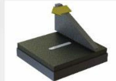
Long, thinner parts with rounded ends will build well, as they also provide a smooth lead in for the blade and are inherently stiff. However, all these issues need to be considered in parallel with the other limits (build angles, etc) mentioned elsewhere in this section.
