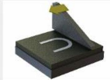
An open 'U' or similar shape is also ideal, as the lead in for the blade is again rounded, and the basic profile will be strong as it builds, resisting the force of the recoating blade.
