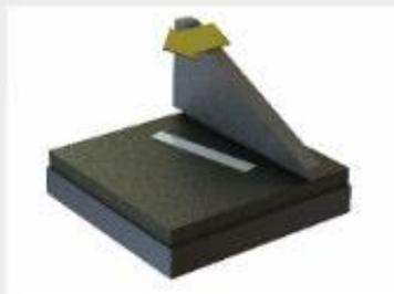
Any flat surfaces need to be at least 5 degrees from parallel with the blade to allow the blade to touch the part at a point, not a face
