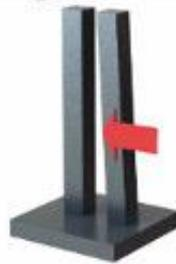
The exact proportions will always depend on the specific geometry, but if the section gets too high, there is a danger that the recoater blade will bend the part, and possibly damage itself in the process, terminating the build sequence.
