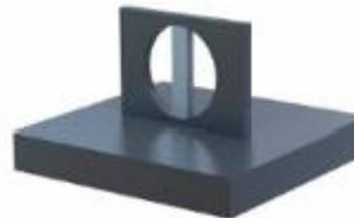
Large holes will require support structures to be added in the centre to prevent the part collapsing or becoming distorted during the build process. These supports will need to be removed by wire cutting or machining
