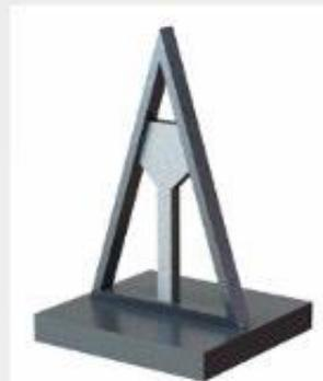
This kind of structure may need a simple support structure up the middle to provide some rigidity before the part is completed.
