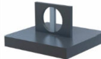
Large holes will require support structures to be added in the centre to prevent the part collapsing or becoming distorted during the build process. These supports will need to be removed by wire cutting or machining
