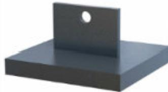
Small holes can be accommodated easily. Holes of less than 6mm diameter are ideal
