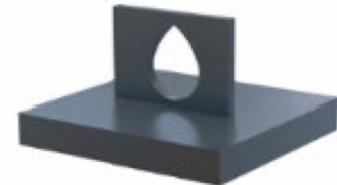
If the hole has an angled or arched upper area it will probably not require any supports. This is one of the features of DMLS that can have a significant impact on the design process
