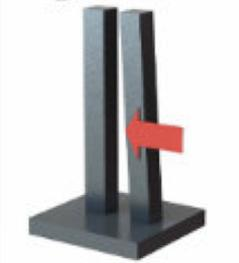
The exact proportions will always depend on the specific geometry, but if the section gets too high, there is a danger that the recoater blade will bend the part, and possibly damage itself in the process, terminating the build sequence.
