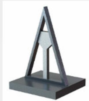
This kind of structure may need a simple support structure up the middle to provide some rigidity before the part is completed.
