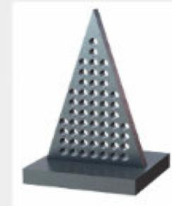
If the reason for the open structure is simply weight reduction, it may be easier to perforate it with holes (ideally less than 6mm in dia) that will reduce weight, but not require any supports.
