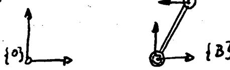
$$\overset{\circ}{A}_2 = T_2(x, D) R(q_5) T_2(x, d_2) R_{\text{rot}}(q_4) = \begin{pmatrix} C_{45} & -S_{45} & D + d_2 C_5 \\ S_{45} & C_{45} & d_2 S_5 \\ 0 & 0 & 1 \end{pmatrix}$$
