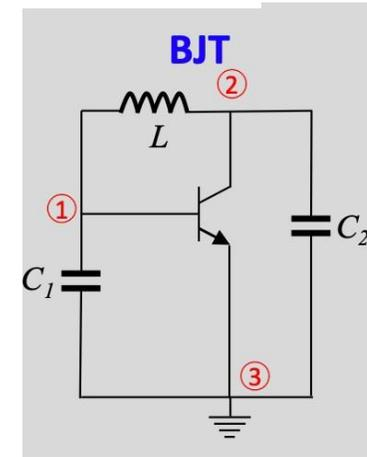
$$-\frac{1}{\omega C_1} - \frac{1}{\omega C_2} + \omega L = 0 \quad \text{con} \quad C = \frac{C_1 C_2}{C_1 + C_2}$$
