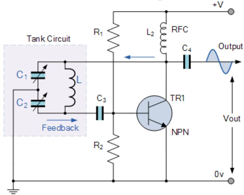
$$\frac{1}{C_T} = \frac{1}{C_1} + \frac{1}{C_2} \quad \text{or} \quad C_T = \frac{C_1 \times C_2}{C_1 + C_2}$$
