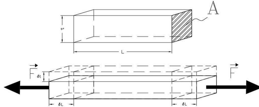
The resistance  $R$  of a conductor of cross section area  $A$ , length  $L$ , made of material of resistivity  $\rho$  is  $R = \rho \frac{l}{A}$
