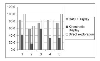
Fig. 7. Percentage of successful recognition of 5 specimens of different softness by direct exploration, and by exploration of two artificial replicae of their proprioceptive and CASR behaviours, respectively.
