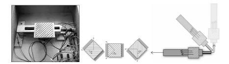
**Fig. 1.** Experimental apparatus for experiment 1: physical appearance (left); changing the pad texture orientation (middle); changing the slide orientation (right).
