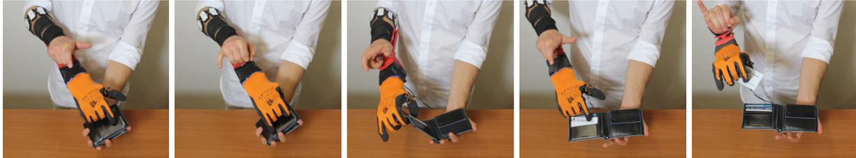
Fig. 11. Bi-manual task consist of open a wallet and grasp a credit card performed by switching between different postures of the hand.
