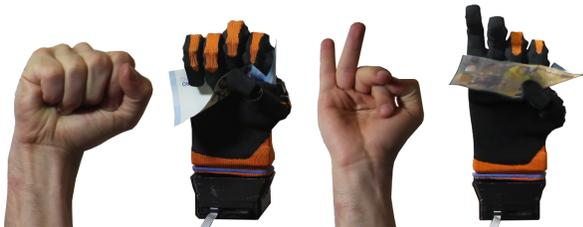
Fig. 9. An example of power and pinch grasp of a banknote. The similarity between the posture of an operator’s hand and the Pisa/IIT SoftHand 2 highlights the simplicity of this control strategy.
