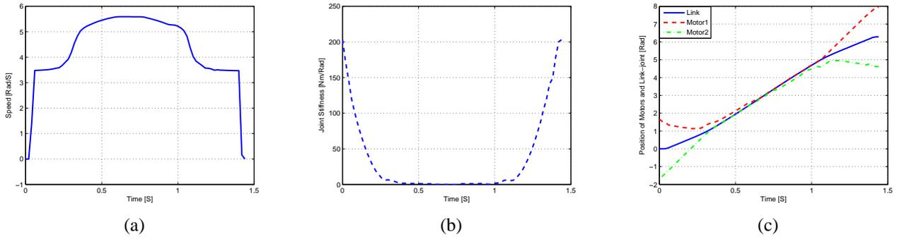
Fig. 4. Optimal operation of simple AA. (a) Link-joint speed, (b) Link-joint stiffness and (c) Motors and Link-joint positions.
