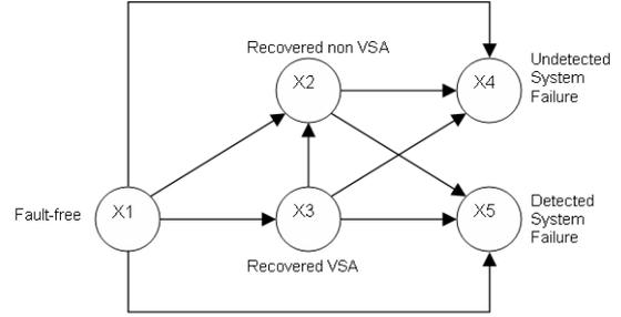
Fig. 3. The general state transition diagram.
