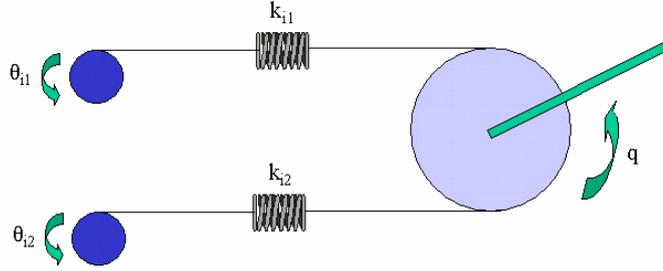
**Fig. 5.** Appearance of an antagonistic VST actuation system for the  $i - th$  joint of a robot arm. The action of the two motors  $\theta_{i1}, \theta_{i2}$  generates a compression or a decompression of springs with nonlinear elasticities  $k_{i1}, k_{i2}$ , allowing the independent variation of joint positions  $q$ , and transmission stiffnesses  $\sigma(q, \theta_{i1}, \theta_{i2})$ .
