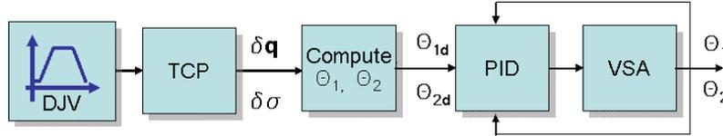
**Fig. 6.** VSA Control System. Desired main shaft positions  $\theta_{1d}, \theta_{2d}$  are chosen accordingly to (1) where  $\delta\sigma$  is computed by the Trajectory Compliance Planner (TCP, [2]) so as to guarantee safety during motion with respect to a desired pre-planned joint velocity (DJV).
