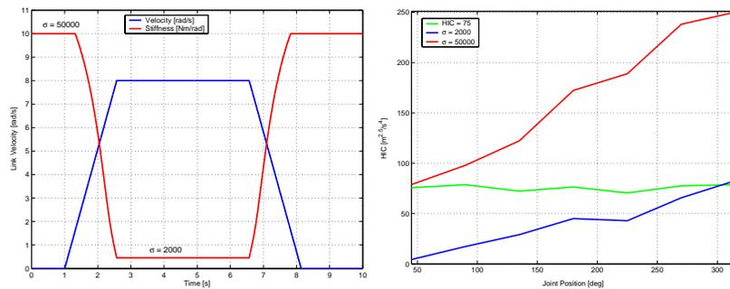
**Fig. 13.** (Left) Output of the TCP for a desired joint velocity at constant safety bound  $HIC = 75$ . The desired stiffness trajectory is obtained by interpolation of results in fig.12. (Right) Impact results in case of rigid (red), compliant (blue), and VIA (green) transmissions related to the accelerating phase of the task.
