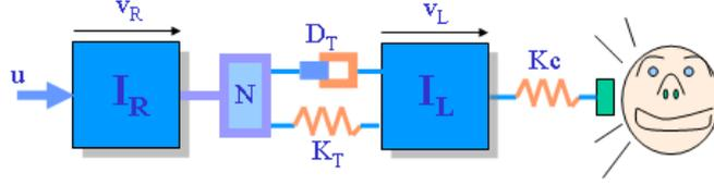
**Fig. 1.** General design of the coupling between torque source and link for a manipulator impacting with human.  $N$  denotes the reduction ratio,  $I_R$  the axial rotor inertia;  $I_L$  is the link inertia at the impact point;  $K_c$  is the effective cover stiffness.
