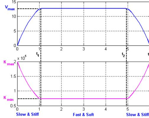
**Fig. 3.** Illustrating the intuitive behaviour of a Variable Stiffness Transmission in a 1DOF rest-to-rest task. High impedance is imposed at low velocities, while low impedance is used at high velocities to reduce potential impact injuries.
