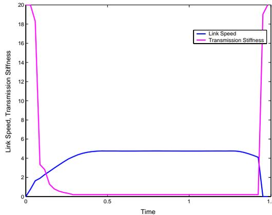
**Fig. 4.** The solution found with the Safe Brachistochrone algorithm for VDA. The minimum time optimal control sets high values of damping (i.e. impedance) for small values of speed and vice versa.
