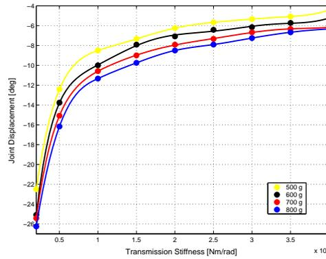
**Fig. 9.** Experimental displacement of the joint shaft of the VSA with respect to the transmission stiffness at increasing values of the applied axial load (from *yellow* to *blue*).
