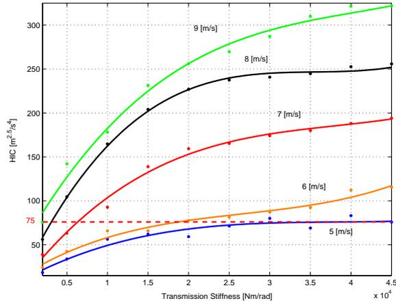
**Fig. 12.** Experimental results of the injury risk in case of impact at different transmission stiffnesses for VSA. As expected, the maximum allowable velocity  $v$  of the joint shaft decreases as the value of transmission stiffness  $\sigma$  increases, if an acceptable level of injury risk is chosen (as e.g the red dashed straight line, corresponding to  $HIC = 75$ ). Continuous lines represent the fourth order minimum square interpolation of the experimental data (dots).
