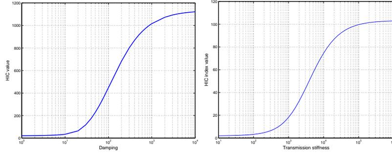
**Fig. 2.** Variation of the injury coefficient HIC (see e.g. [7], [1], [3]) for system in fig.1 with respect to impedance parameters, at constant link velocity  $v = 2 [m/s]$ , and rotor and link inertias  $M_{rot} = M_{link} = 1 [Kg]$ . As expected, in case of impact the injury risk increases with the coupling between the rotor and link.
