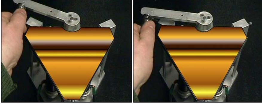
**Fig. 7.** The VSA developed at the Centro Interdipartimentale di Ricerca “E. Piaggio”. The actuator is designed to allow the independent control of joint shaft position and stiffness (see the VSA in compliant (*left*) and stiff (*right*) configurations).
